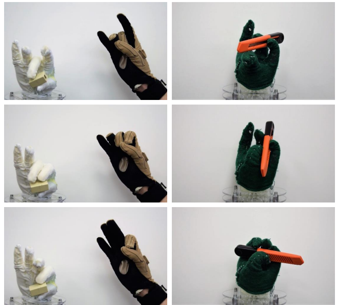
Fig. 3. Left) Telemanipulation sequence of a small cuboid executed by a human operator using the CyberGlove and the trained regression model. Right) Open-loop controlled manipulation sequence created by interpolating between tendon actuation keyframes.
