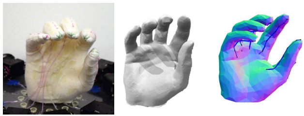
Fig. 8. Anthropomorphic foam hand prototype in its rest pose. Left) physical foam hand prototype, Middle) Scan of the prototype, Right) Finite element mesh used in simulation.
