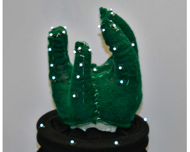
Fig. 5. Four-fingered hand with Vicon markers.
